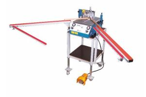
The Jumbo cramp – edge connecting machine is available as automatic and manual version. With a 90° support and two clamping cylinders one from the top one from the front. Each cylinder has a separate pressure control. Through the electronic control you can place cramps behind and on top of each other into glass ledges. The Cramping device can be mounted on a work bench with a glue spreader. The RU-KEV is operated manual and/or by a foot valve.
